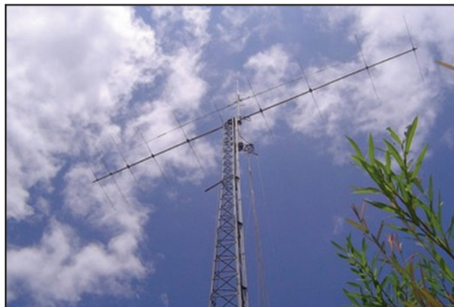
JA6WFM used this big 10-element Yagi on 6 meters to again lead all scorers in Japan. Besides working JAs, Hiro also worked HS, XV9, BM, and VR2.
