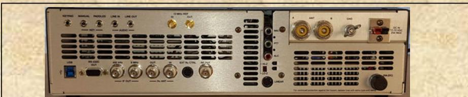
Elegant back panel provides PC interface, keypad input, paddles and manual key inputs, two IF outputs for panadapters, Rx line-out, Rx and Tx line-in, Rx and Tx band data, 20mW transverter output, ALC input, PTT, linear control, Hi/Lo-Z mic switch, 10 MHz ref in and out, main antenna A/B, ground lug, APP DC input, 100W amp fuse.
