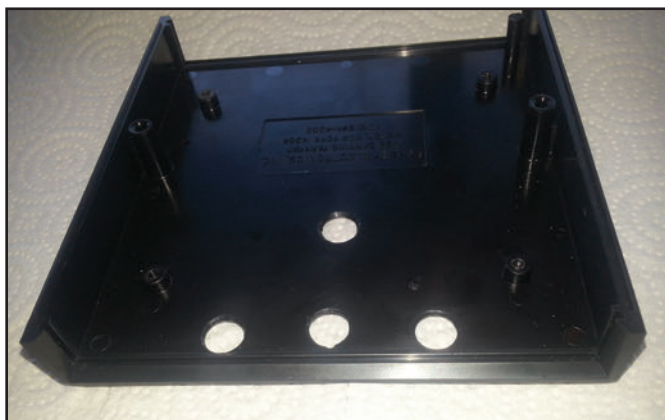
Photo G. Holes on the bottom of the Ramsey amplifier's enclosure allow air to flow through the cabinet interior, helping to keep the final RF transistors cool.
